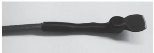
Do not subject the thermostat to mechanical stress. Attach the flat side of the thermostat to the **cold water pipeline**.
